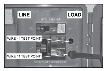
Figure 4. Test 7 Test Points
